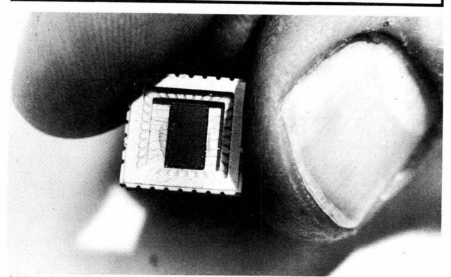
SANDIA WILL PRODUCE 11,000 RADIATION-HARDENED microprocessors, memories and custom-integrated circuits for use in NASA's upcoming Galileo and Solar Polar space programs. The package is approximately half an inch square with a silicon gate memory that can store up to 1000 bits of information. (See story on Page 5.)
